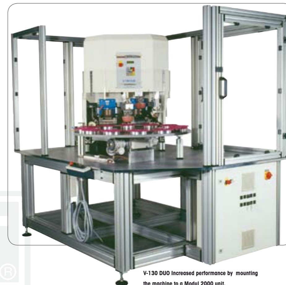
V-DUO with ink residue pick-up system (included)
