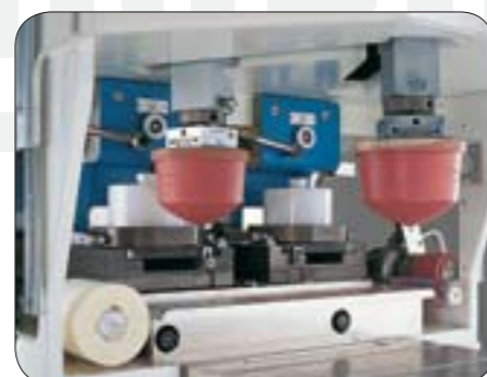
right tampon in the front prints, left tampon in the rear
