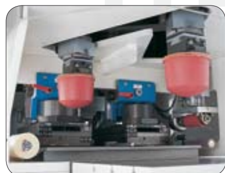
V-shaped arrangement of the 2 printing units
