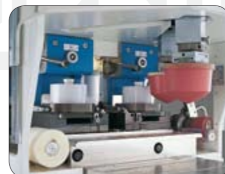
left tampon in the front prints, right tampon in the rear
