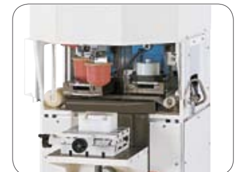
V-DUO with printing component on x-y cross table (option)
