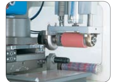
V-DUO with ink residue pick-up system (included)
